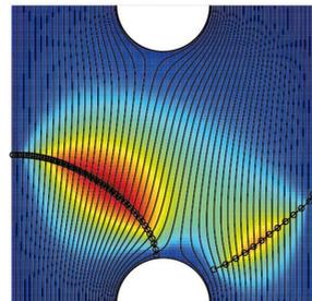
Figure 2. Buffer beam. Black lines are voltage without space charge; color regions are the perturbation.
