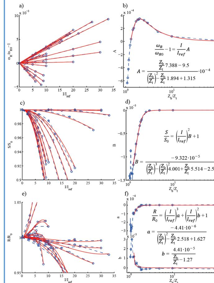
Figure 4. Changes in performance for different  $I/I_{ref}$  and  $Z_b/Z_t$ : a), b) resonant frequency; c), d) peak signal; e), f) resolving power.
