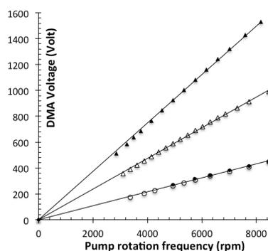
Figure 4: Blower response given as mean peak voltage versus rotation frequency  $V_{DMA}(\omega)$  obtained for three different flow restrictions inserted in the closed circuit. Because  $Q \sim V_{DMA}$ , the data validate Equation (6) at  $\omega > 4000$  rpm.
