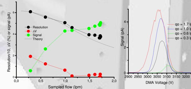
Figure 5a - Effect of sampled flow on total transmitted THA+ signal, peak resolution and THA+ classification voltage ( $\Delta V$ , deviation from the 3055 V at which THA+ signal is maximum at maximum sampling rate),
