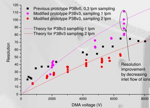
DMA prototype modified for coupling to Shimadzu's 1 lpm sampling single quad
