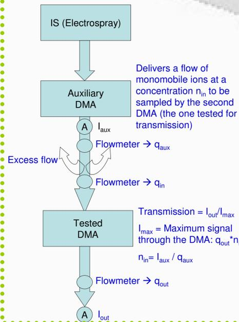
Figure 2 - Transmission tests for DMA model P4, which samples  $q_{out} = 0.8$  lpm
