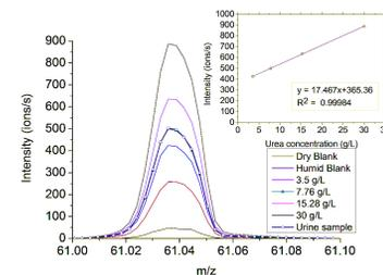
**Figure 3.** Urea peak measured from urea solutions in water and from a urine sample. Note also the signal increase when moisturizing the ambient air. The inset shows the corresponding calibration curve with a detection limit of ~ 2 g/L. The inferred urea concentration in urine is ~ 7.8 g/L (37 ppt in vapor phase for an ideal solution).
