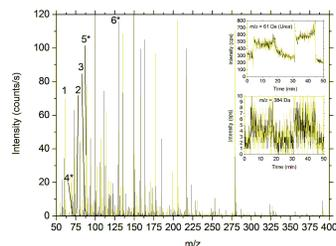
**Figure 2.** Positive urine spectrum (blank subtracted). The inset shows the corresponding single ion monitoring (SIM) trace for urea (top) and for the heaviest vapor clearly seen at 384 Da. The steps are produced when placing the urine sample close to the entrance of the ionization chamber. 1: Urea; 2: Amino-2-propanol; 3: Piperidine; 4\*: 1-Pyrroline; 5\*: 4-Aminobutanol; 6\*: octylamine.\*Compounds tentatively identified.
