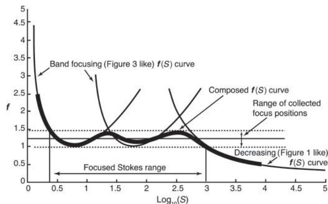
FIG. 2. Schematic of the  $f(S)$  curve for particles accelerated first through a contraction with  $d \gg 1$ , and then through 2 additional contractions having  $d$  values comparable to unity.
