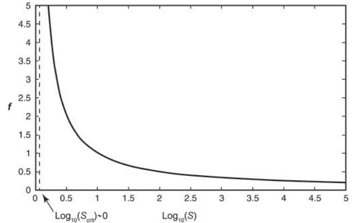
FIG. 1. Schematic dependence  $f(S)$  of the focal distance  $f$  (normalized with the nozzle throat diameter) on the Stokes number  $S$  for particles accelerated through a focusing contraction with  $d \gg 1$ .
