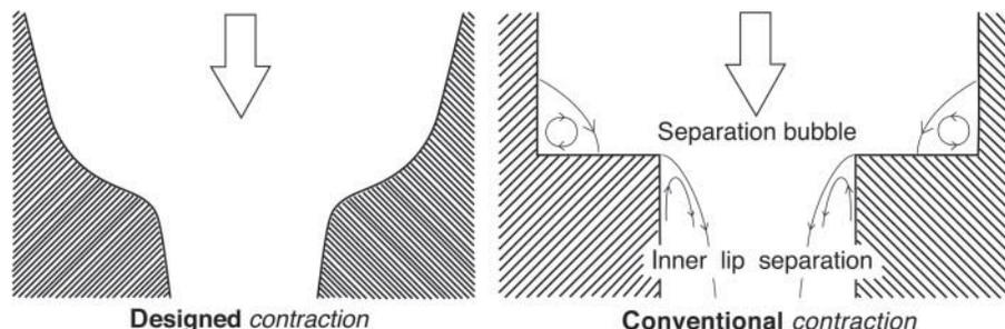
FIG. 3. Section of an individual focusing *contraction*. Right: conventional contraction subject to the appearance of a separation bubble at the outer corner, and flow separation at the inner lip. Left: well designed *contraction* avoiding these 2 problems.
