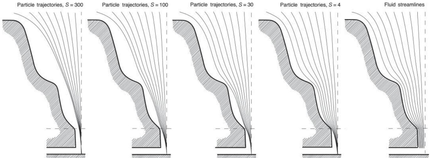
FIG. 7. Meridional section of a composite focusing nozzle formed by a series of 3 axisymmetric *contractions*, and capable of focusing a wide range of particle sizes in the same region at high *Re*.  $S = 300, 100, 30, 4$ , and streamlines, from right to left.
