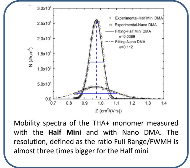
Mobility spectra of the THA+ monomer measured with the **Half Mini** and with Nano DMA. The resolution, defined as the ratio Full Range/FWHM is almost three times bigger for the Half mini
