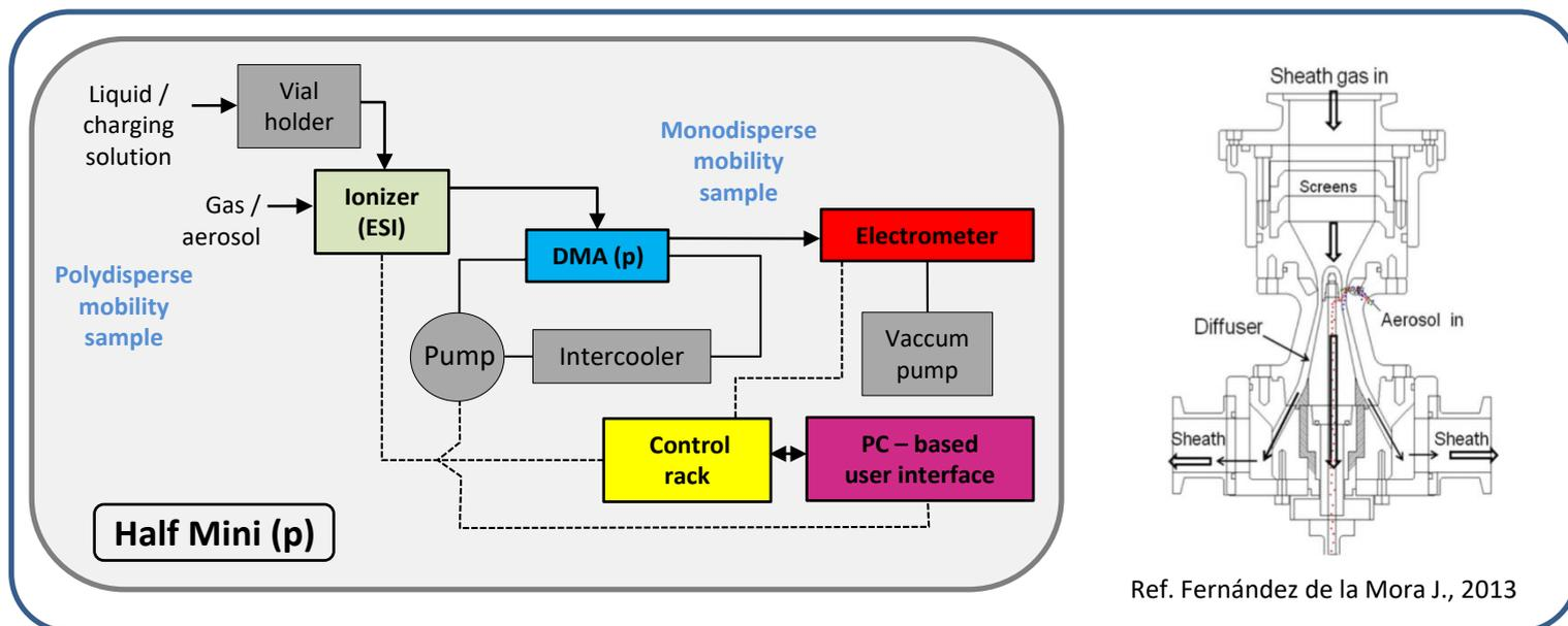
In the **Half Mini** system, the molecules or particles are ionized in an electro-spray ionization chamber and then submitted simultaneously to a gas flow and an electric field within the cylindrical **Differential Mobility Analyzer (DMA)**. Only the particles or ions with a specific mobility are transmitted into the DMA outlet.
