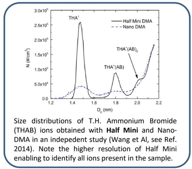
Size distributions of T.H. Ammonium Bromide (THAB) ions obtained with **Half Mini** and Nano-DMA in an independent study (Wang et Al, see Ref. 2014). Note the higher resolution of Half Mini enabling to identify all ions present in the sample.
