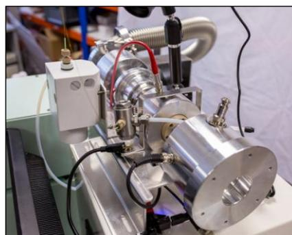
Figure 1. The high temperature capable half-mini DMA.
