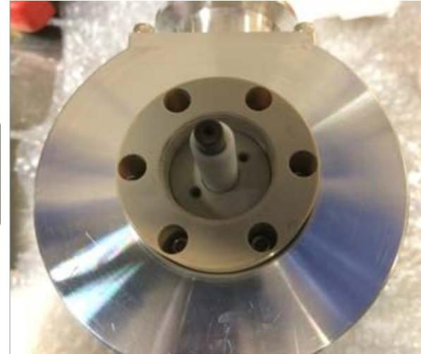
The static dissipative polyurethane tube was substituted with a resistive glass capillary (581 MegaOhms, Photonis, USA).
