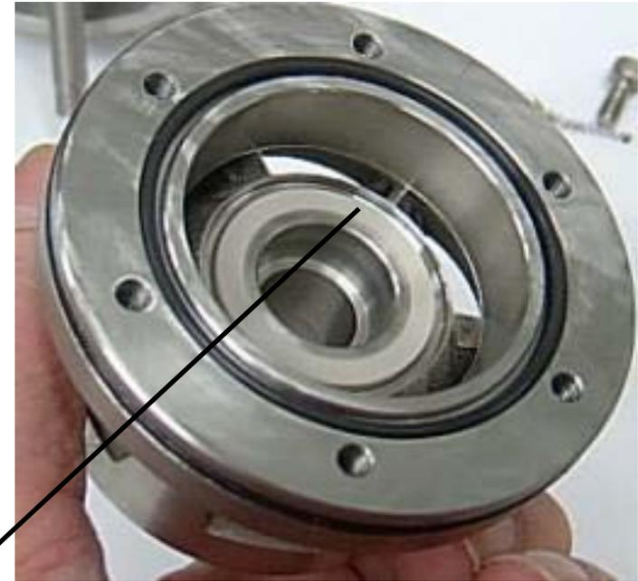
Metal-PEEK-metal sandwich for precision centering of inner electrode
