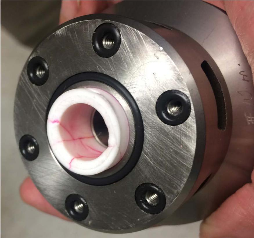
**Macor:** Indeed cracks become visible after coloring and washing,
